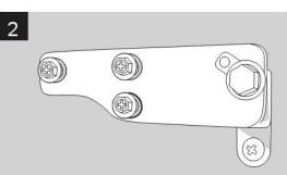
Remove the screws and bracket. Place to one side.
